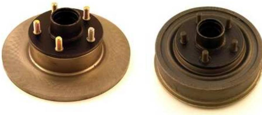
Don't separate the drum or rotor from the hub. If you do, we will not accept the core.
