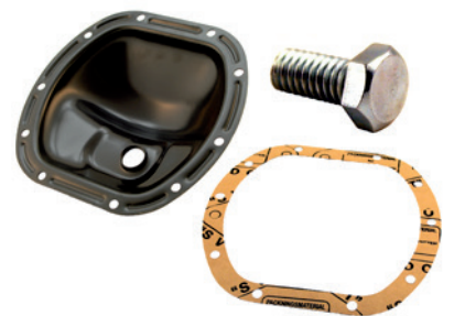
A13/14/16 Inspection cover/gasket/bolt
