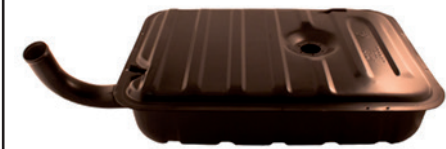
A1 Fuel tank
